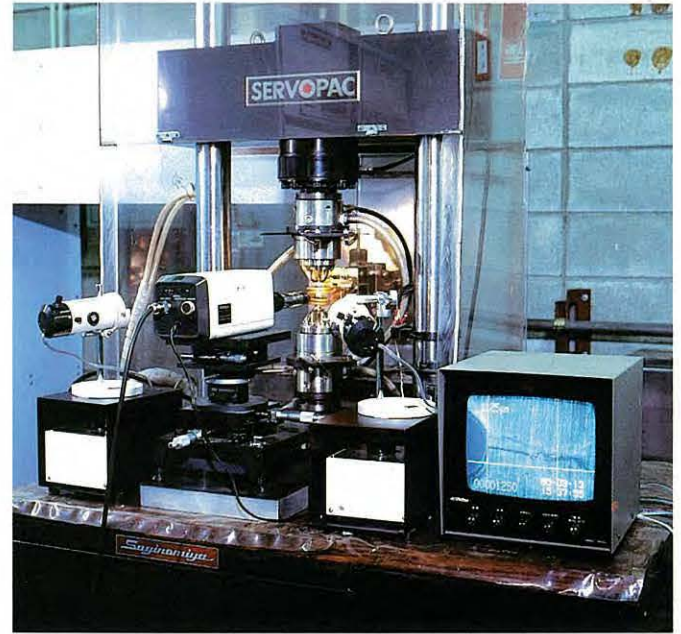
Fatigue crack propagation test of turbine blade material at elevated temperatures
